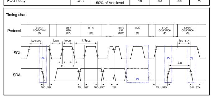
When accessing this device, all communication from transmitting the start condition to transmitting the stop condition after access should be completed within 0.95 seconds. If such communication requires **0.95 seconds** or longer, the I<sup>2</sup>C bus interface is reset by the internal bus timeout function.
